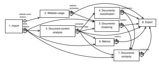
Fig. 3. General workflow of the IIF. Thick arrows correspond to outputs of workflow nodes, thin arrows correspond to connections between inputs and outputs.
